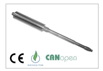
The KD Series are for use in high temperature applications where the process temperatures may reach 538°C (1000°F) such as high temperature engineered polymers. The K Series utilizes standard melt pressure principles and construction, but uses a near incompressible NAK (Sodium Potassium) for pressure transmission. The K Series strain sensing technology is thick film on Stainless Steel.
