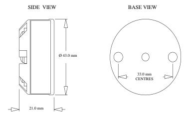
Fixing holes 2 x Ø5.5 mm, Centre hole Ø4.5 mm
