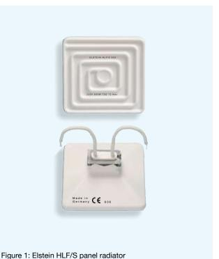
Elstein HLF/S panel radiators are ceramic infrared radiators, which can be used for operating temperatures up to 750 °C and surface ratings up to 64 kW/m².
