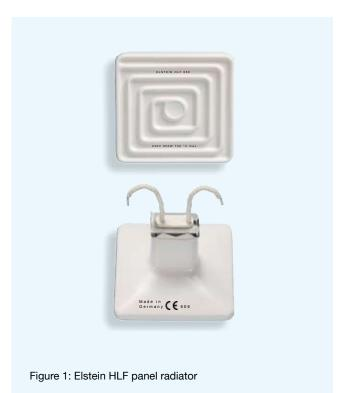
Elstein HLF panel radiators are ceramic infrared radiators, which can be used for operating temperatures up to 700°C and surface ratings up to 42 kW/m².
