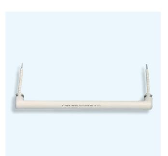
Elstein IRS/330 rod radiators are ceramic infrared radiators with operating temperatures up to 750 °C and surface ratings up to 36 kW/m<sup>2</sup>. They have one mounting socket on each side, with witch they can be fixed to a mounting sheet with fixing springs.
